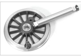
proud of the wheel back. I then fill the countersink hole with Araldite and then screw it in until it locks. Leave the wheels until the Araldite has set and then clean of any excess Araldite by rubbing the wheel on the emery cloth. This should leave the screw head embedded in Araldite and prevent the potential problem of the screw turning when you are trying to undo the crankpin nut.
