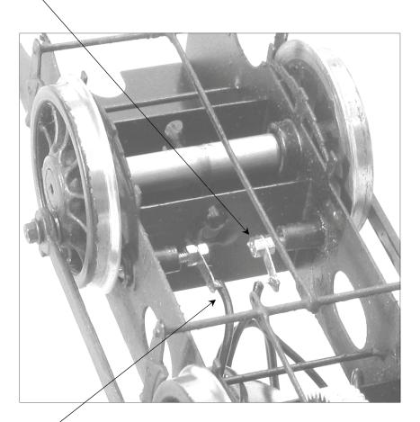
Also note how the electrical wire is gently curved so as to allow movement of the pickup
