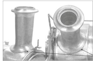
The chimney has been soldered into place with a generous fillet of 70° solder run around the base. Then using a curved scalpel blade the excess solder has been scraped back from the brass smokebox and a fibreglass brush worked around the base of the flange to reveal a distinctive circular edge to the casting and feathering the solder into the brass.
